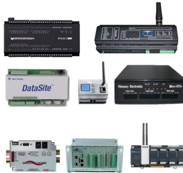
RTUs (Remote Terminal Unit)
