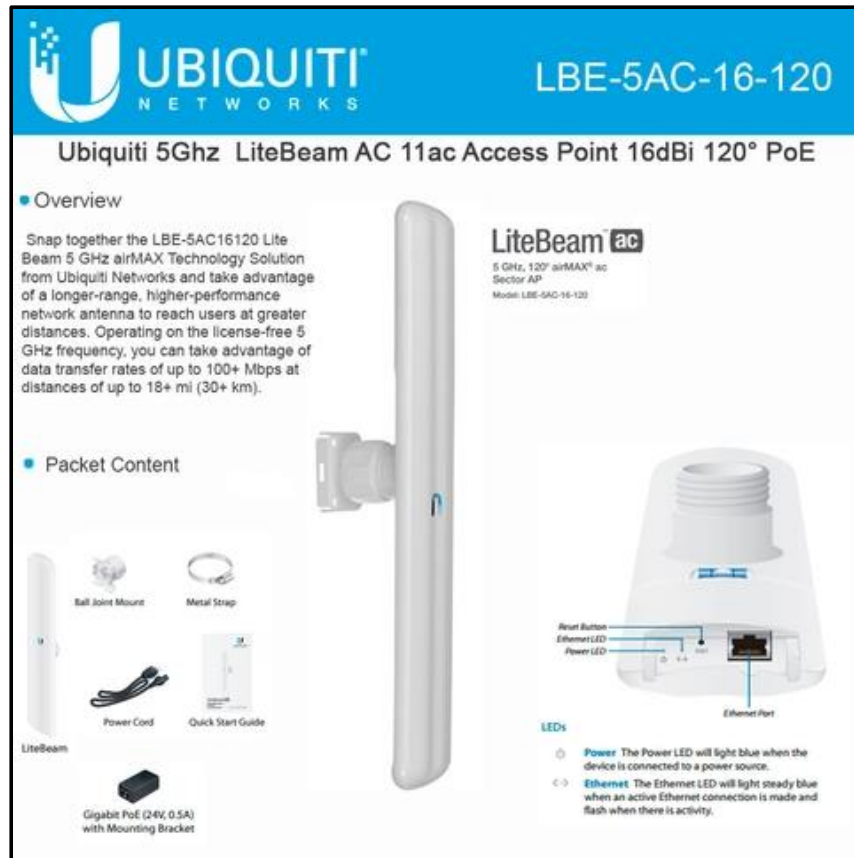
Figura 19. Antena AP LiteBeam AC Modelo: LBE-5AC-16-120
