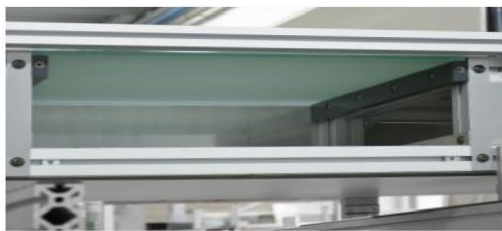
Scratch-resistant glass panel as belt running surface in the lighting area
