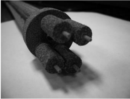
Example of dirty measuring electrodes
