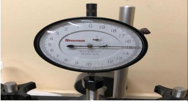
A close-up photograph of a dial used for measuring vertical displacement during a consolidation test. The dial is circular with a scale from 0 to 19. The needle points to approximately 15. The brand name 'Storven' is visible on the dial. |
