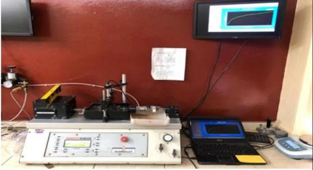
A photograph of a laboratory setup for a direct shear test. It includes a shear box, a normal load frame, and a force-measuring device. A laptop is connected to the equipment, and a monitor displays a graph. The background is a red wall.   |
