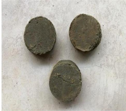
A photograph showing three circular soil samples, likely prepared for direct shear tests. The samples are dark brown and appear to be made of soil with varying textures, consistent with the description of silty sand and silty sand soil. |
