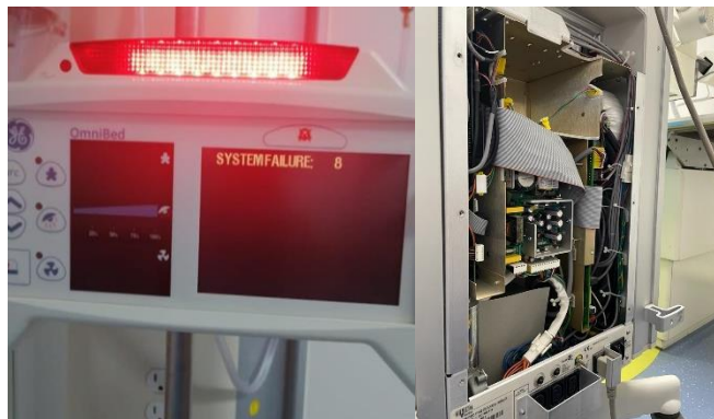
Ilustración 27- Incubadora General Electric Giraffe® OmniBed "SYSTEM FAILURE: 8".
