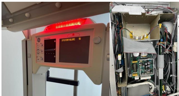
Ilustración 28- Incubadora General Electric Giraffe® OmniBed "SYSTEM FAILURE: 15".
